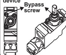
**Valve without flame failure device**
